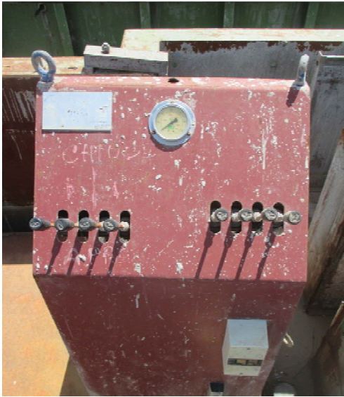
Oleo-dynamic control unit (sole to command the 2 formworks 26 meters long)
